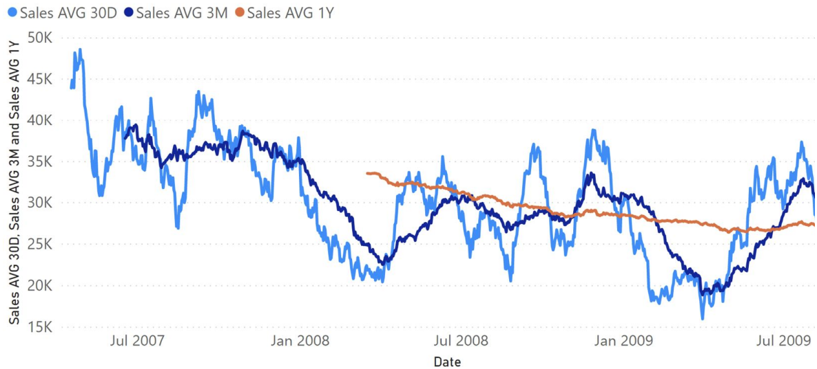
FIGURE 5-17 Sales AVG 30D , Sales AVG 3M , and Sales AVG 1Y show the moving average over 30 days, three months, and one year, respectively.
